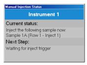
2 The dialog will always specify the sample (sample name) which shall be injected, thus mistakes will be prevented if multiple samples are to be injected within the same sequence.
