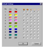
The default calibration settings file located in the program folder (calibration.cfg) contains the information on the view and number of displayed columns, color scheme for data points as well as the color scheme and captions of the axis. Upon loading a setting file all parameters will be updated and overwritten if not saved previously.
