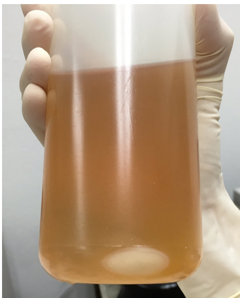
Figure 9 0.5-L centrifuge bottle with visible pellet of E. coli cells harvested from 330 mL of solution from an amplification bottle ( \sim 1/3 of the bottle) in a Beckman JA-10 fixed-angle rotor
