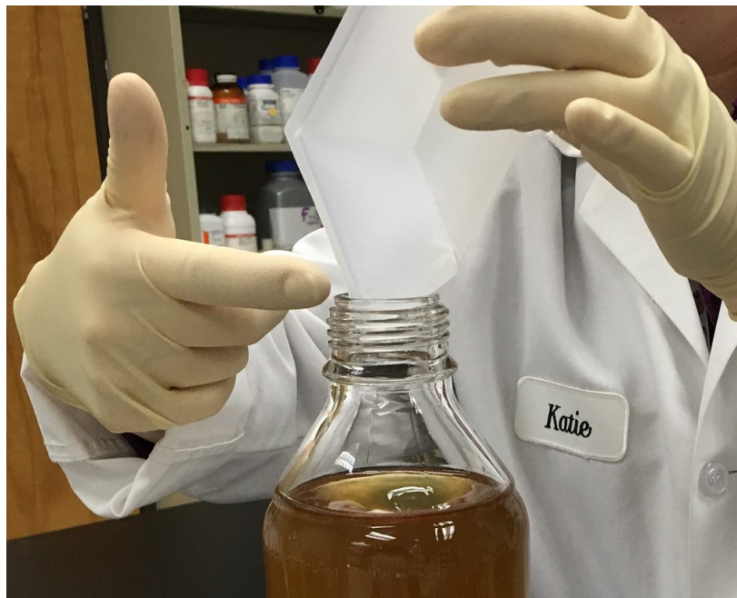
Figure 4 Technique for slowly adding agarose to an amplification bottle
