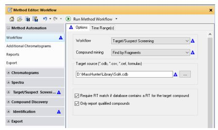
5 In the Method Editor, click **Target/Suspect Screening > Find by Fragments** and click the **Target Source** tab.
