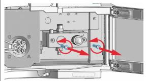
7 Remove the pump head from the pump drive.
