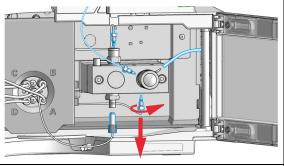
**6** Using a 4 mm hexagonal key, stepwise loosen the two pump head screws.
