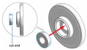
**13** *G5654A only*: Place a seal wash gasket in the recess of the support ring. Use a matching orientation of gasket and support ring. Put the seal holder on top of the gasket.
