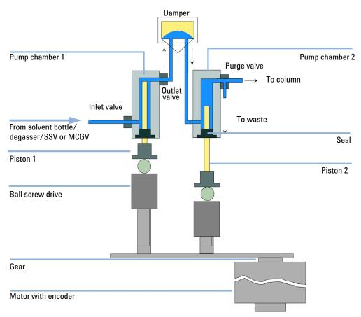
Figure 8 Principle of the Pump
