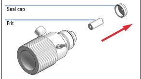
4 Using a pair of tweezers or a toothpick remove the frit.
