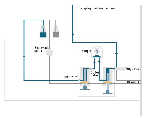
Figure 6 Hydraulic path of the isocratic pump
