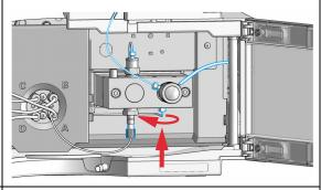
5 Reconnect the valve capillary to the outlet valve.
