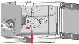
7 Reconnect the outlet capillary and the waste tubing.
