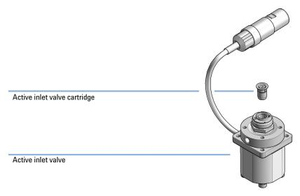
Figure 17 Active Inlet Valve Assembly
