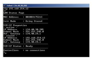
change of IP setting to Initialization mode is Using Stored
