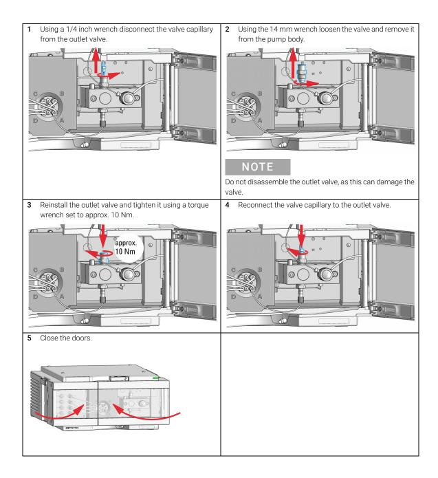
Exchange the Purge Valve Frit or the Purge Valve
