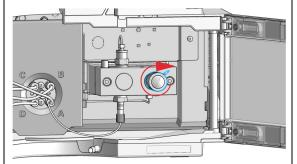
8 Reconnect the outlet capillary and the waste tubing.
