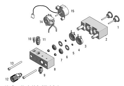
Figure 14 Pump Head with Seal Wash Option
