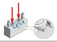
Maintenance of a Pump Head with Seal Wash Option
