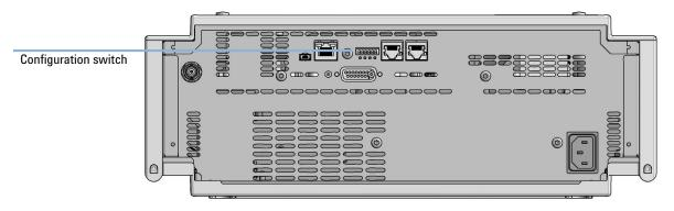
Figure 26 Location of Configuration switch (example shows a G7114A/B VWD)
