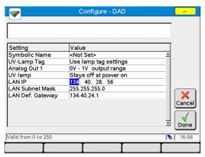
Figure 38 Instant Pilot - LAN Configuration (Edit mode)
