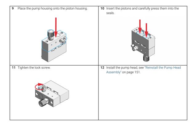
Maintenance of a Pump Head with Seal Wash Option
