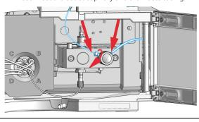
8 If installed, reconnect the active inlet valve cable to its connector.
