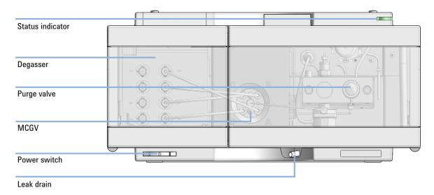
Figure 5 Overview of the Bio-inert Pump
