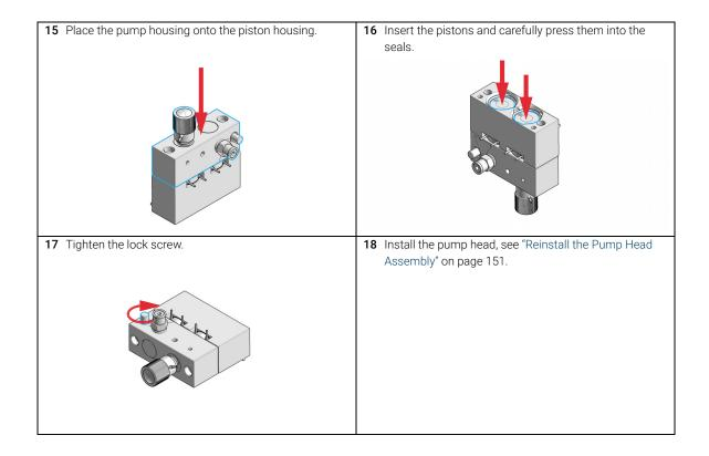
Reinstall the Pump Head Assembly
