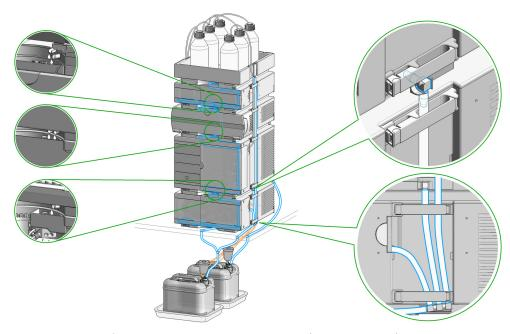
Figure 10 Infinity II Single Stack Leak Waste Concept (bench installation)
