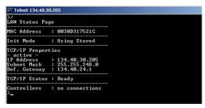
Figure 35 Telnet - Current settings in "Using Stored" mode
