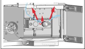
4 If applicable, remove tubings from the seal wash support rings.
