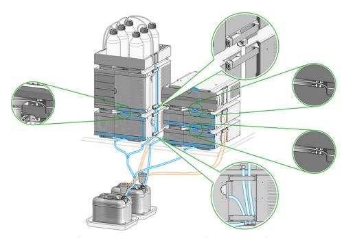
Figure 11 Infinity II Two Stack Leak Waste Concept (bench installation)
