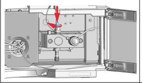
6 Reconnect the solvent inlet tube to the passive inlet valve.
