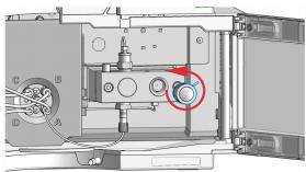
3 Remove the seal cap from the purge valve.
