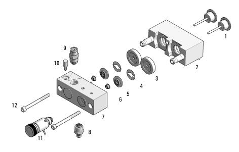
Figure 13 Pump head assembly without seal wash option
