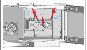
2 Using the 14 mm wrench unscrew the purge valve and remove it.
