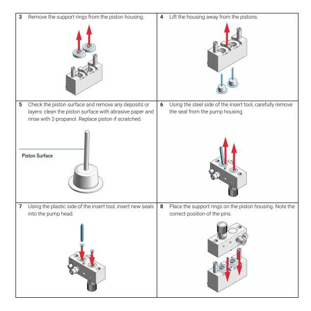
Maintenance of a Pump Head Without Seal Wash Option
