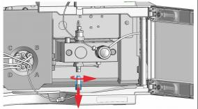
3 Using a 1/4 inch wrench disconnect the pump outlet capillary from the purge valve. Disconnect the waste tube.
