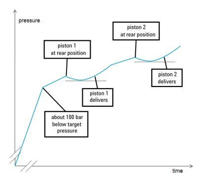
Initially, the pressure is increased to about 100 bar below the target pressure, which has been set for the test.
