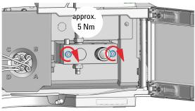
4 Install the capillary at the bottom of the pump head.
