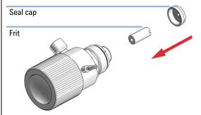
6 Reinstall the seal cap including the gold seal.
