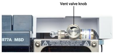
Do **not** turn the knob too far or the O-ring may fall out of its groove. Close the vent valve before pumping down.
