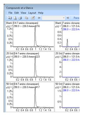
The MassHunter Quantitative Analysis software will quantify very low amounts of sample.
