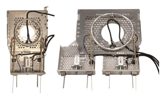
Figure 19 Routing the transfer line heater wires
