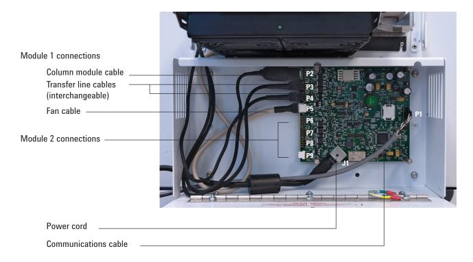
Figure 34 LTM electronics board cable connections
