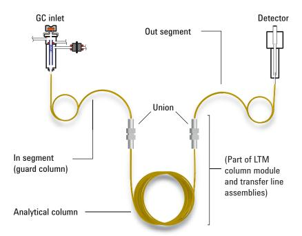
Figure 31 7890A GC Composite column parts
