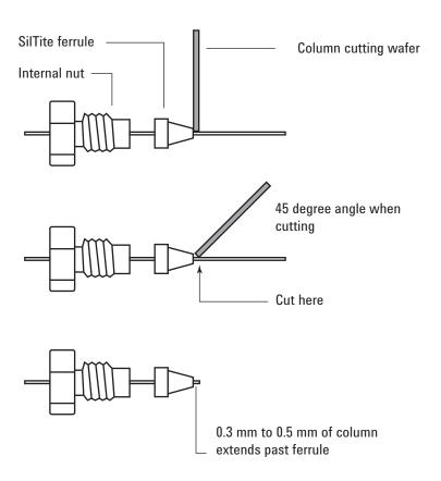
Figure 11 Technique for trimming the column in a CFT fitting
