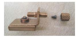
Start by observing the clamps with the mini-unions. The screw on each of these can be loosened just enough that the brackets can slide along the rails projecting from the oven-side of the transfer line module. It is not necessary to remove the screw; just loosening the screw will allow the bracket to slide on and off of the rail.
