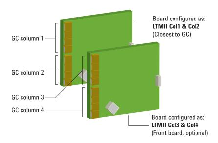
Figure 27 7890A GC column assignments by electronics board position
