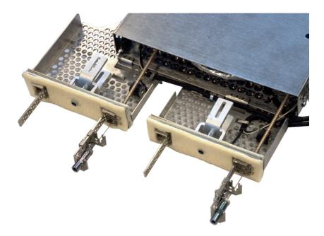
Figure 23 Gaskets installed on a 5-inch module assembly
