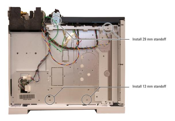
Figure 33 Installing the left side panel standoffs
