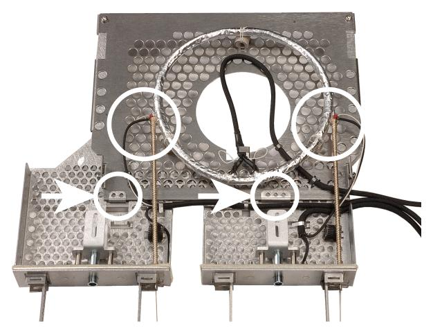
Figure 17 Column module in place on transfer line module (5-inch column module shown)
