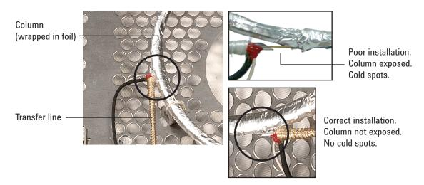
Figure 18 Correct installation of column into transfer line
