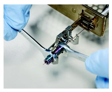
11 After tightening, lift the union from the bracket. Gently pull the column to determine if the swage is secure. If not secure, tighten by no more than 10 ° rotation.
