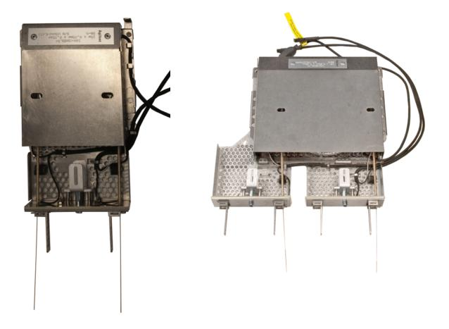
Figure 20 Column modules installed onto transfer line modules
