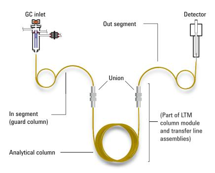
Figure 40 7890A GC Composite column parts
