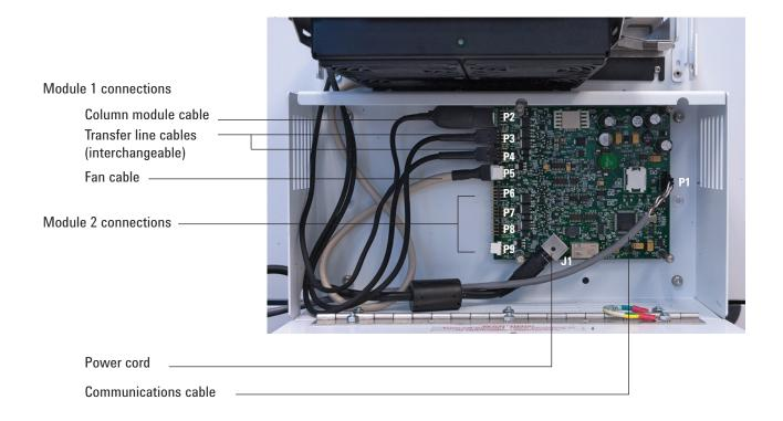
Figure 26 LTM electronics board cable connections
