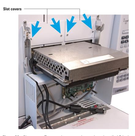
**Figure 36** Slot covers. Two top slot covers shown above installed 5-inch column module.
