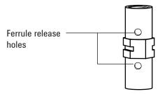
Figure 12 CFT union ferrule release holes
