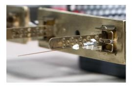
Figure 21 Internal nut and SilTite ferrule on column
