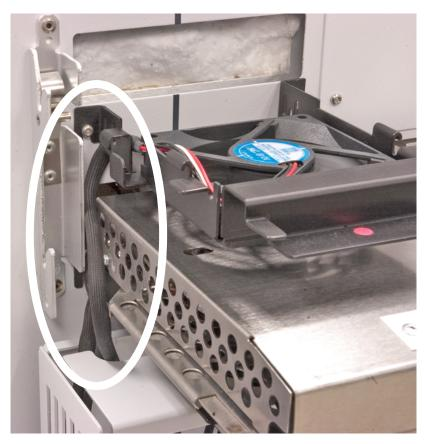
7 Connect the fan cable to the electronics board at P6 (or P9 for module 2). See Figure 34.
