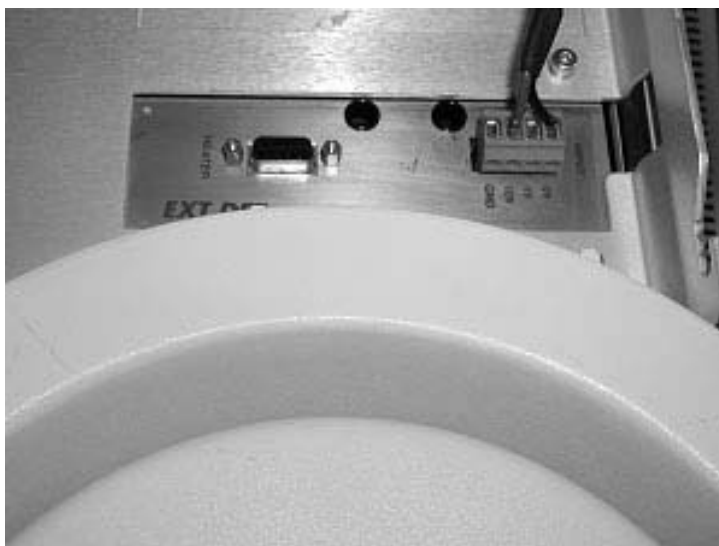
Figure 1 The Signal Cable Connection on the GC
