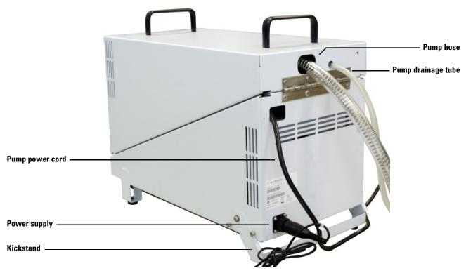
Figure 2 Quiet Cover GC/MS (rear view)
