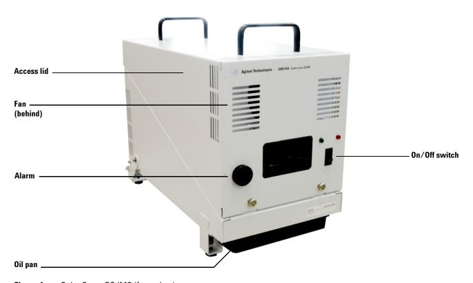
Figure 1 Quiet Cover GC/MS (front view)
