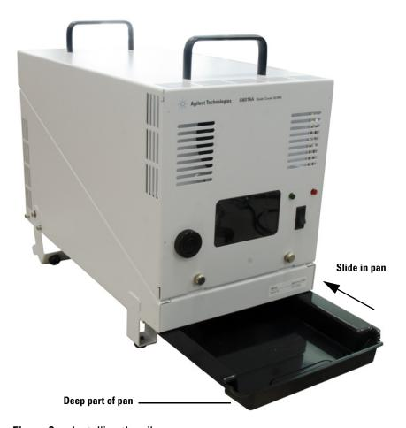
Figure 3 Installing the oil pan
