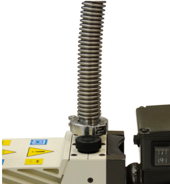
Figure 9 Pump hose connected to the rough pump (DS 302 shown)
