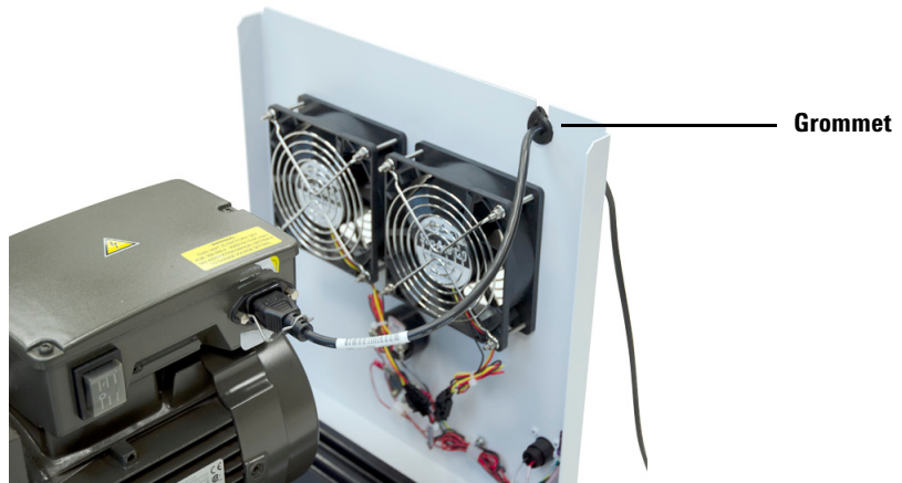
Figure 7 Installed pump power cord (DS 302 shown)
