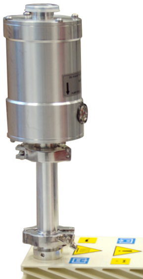
Figure 8 Mist filter attached to rough pump (DS 302 shown)
