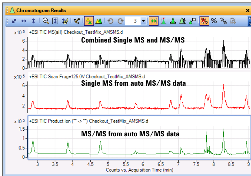
Figure 33 The top chromatogram shows all of the data points for single-MS and MS/MS. MS/MS data points have lower total signal because ions in a narrow mass range are isolated for fragmentation. The middle chromatogram shows the single-MS only and it is clear that the Q-TOF LC/MS is collecting mostly single-MS data. The bottom chromatogram is created by connecting all points where MS/MS spectra were acquired.
