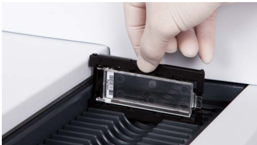
Figure 12 Inserting slide holder into cassette
