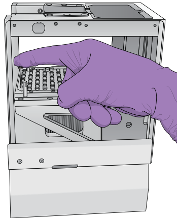
Figure Pushing down on piston rod of replaced syringe
