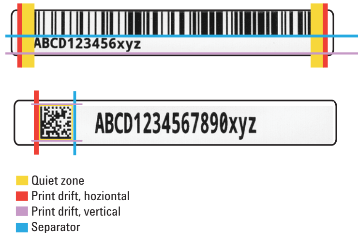
Figure 4 Minimum blank margins for Code 128 (top) and Data Matrix (bottom) symbologies
