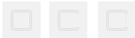
Figure 8 Evaluating the seals of sample wells. L: Good impression, with defined edge of chimney/rim. C and R: Poor impression, with missing or very faint segments.
