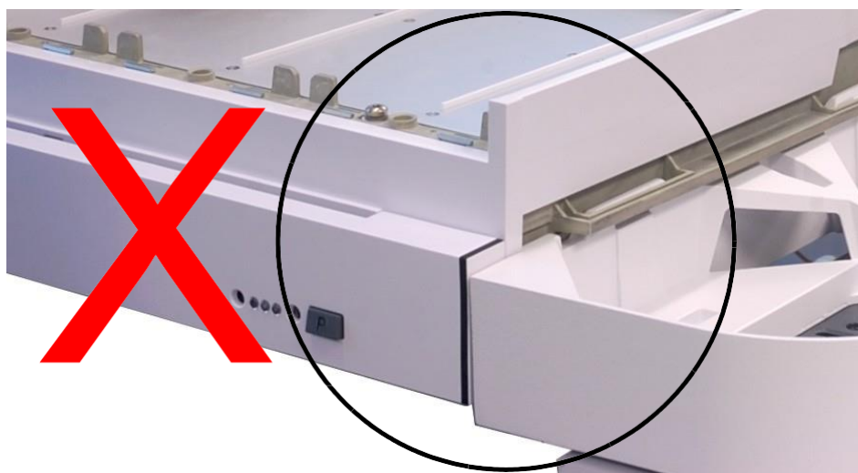
Figure 6. Sample tray incorrectly installed.
