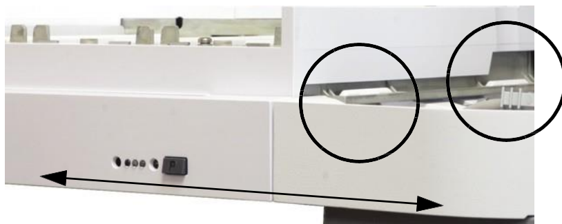
Figure 5. Sample tray correctly installed.
