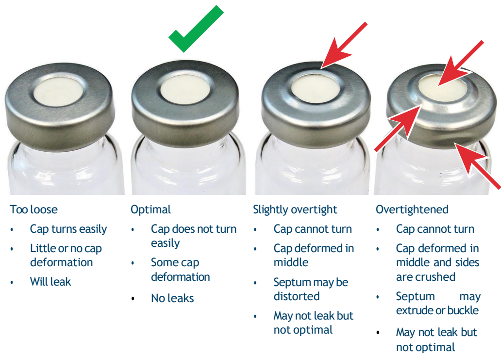
Figure 57. Acceptable and unacceptable vial caps
