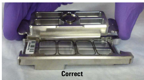
Figure 15. Chamber cover in correct (left) and incorrect (right) orientations
