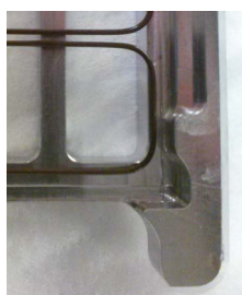
Figure 12. Correct positioning of gasket slide in chamber base
