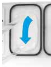
Figure 13. Drag and dispense method – Start dispensing when the pipette tip is near the top of the well. Finish dispensing when the pipette tip is near the bottom of the well.
