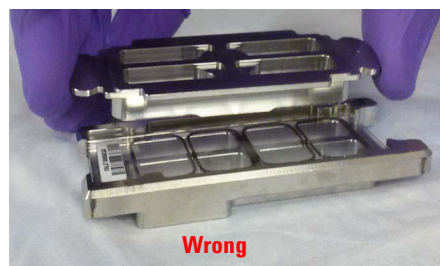
Figure 15. Chamber cover in correct (left) and incorrect (right) orientations
