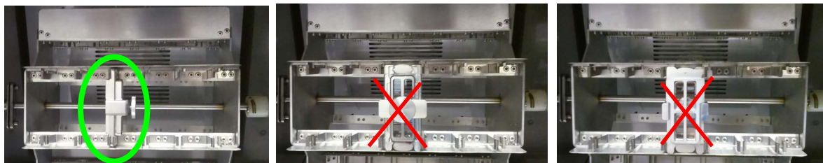
Figure 20. Assembled chambers in correct (left) and incorrect (middle and right) orientations
