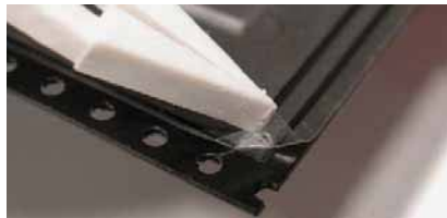
Figure 3. Removal of clear plastic covering
