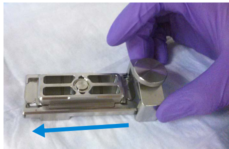
Figure 10. Slipping the clamp onto the chamber base
