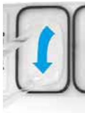
Figure 7. Drag and dispense method – Start dispensing when the pipette tip is near the top of the well. Finish dispensing when the pipette tip is near the bottom of the well.
