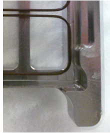
Figure 6. Correct positioning of gasket slide in chamber base
