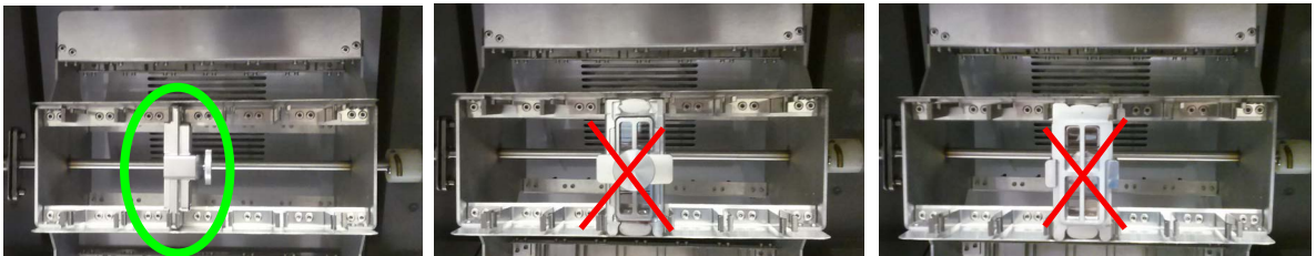
Figure 14. Assembled chambers in correct (left) and incorrect (middle and right) orientations
