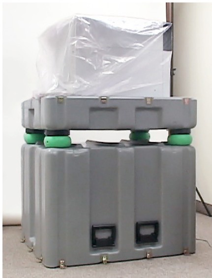
Figure 12 Using the cover to elevate the instrument to operating height
