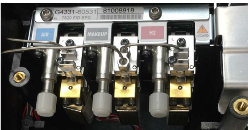
Figure 2 Example EPC flow module with FID tubing attached
