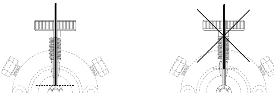
Figure 51 Correct and incorrect Valve Needle Penetration Depth
