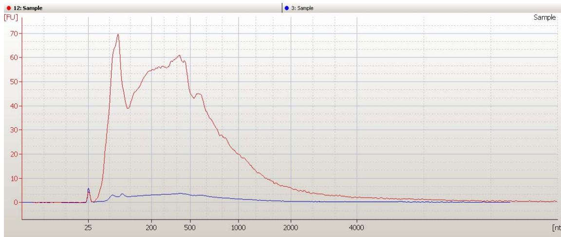
Figure 9 Non-Fragmented cRNA products from Agilent’s Two-Color Microarray-Based Exon Analysis (Low Input Quick Amp WT Labeling kit). Concentration was 160 ng/μL according to NanoDrop. 1μL was analyzed with the mRNA Nano assay. Red, Cy5-labeled cRNA; Blue, Cy3-labeled cRNA showed the same size distribution. Because Cy5 is excited under the 2100 bioanalyzer assay conditions, the Cy5-labeled reagents generate two dominant peaks, the first at 100 nt and the second between 200 to 400 nt. In comparison to Cy3-labeled cRNA, the Cy5-labeled cRNA yields additional fluorescence in the profile for the same reason.
