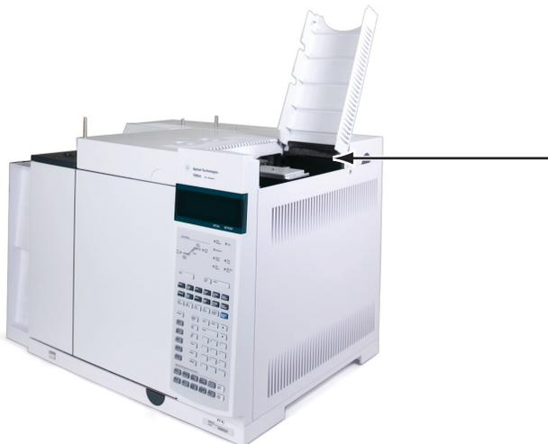
**Figure 2** Lifting the electronics top cover (7890A)
