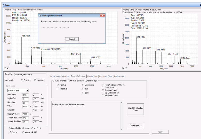
Figure 2 Tune window for a 6530 Q-TOF instrument performing a classic autotune
