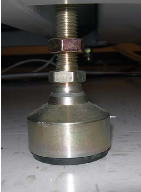
Figure 23 Extend the pump tray feet
