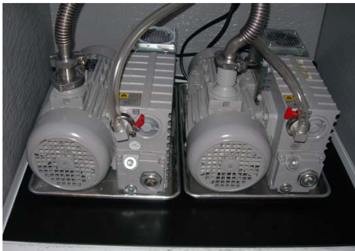
Figure 17 Dual MS40 Pump orientation
