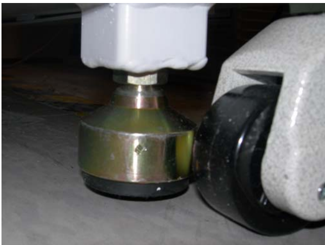
Figure 21 Extending the pump tray feet
