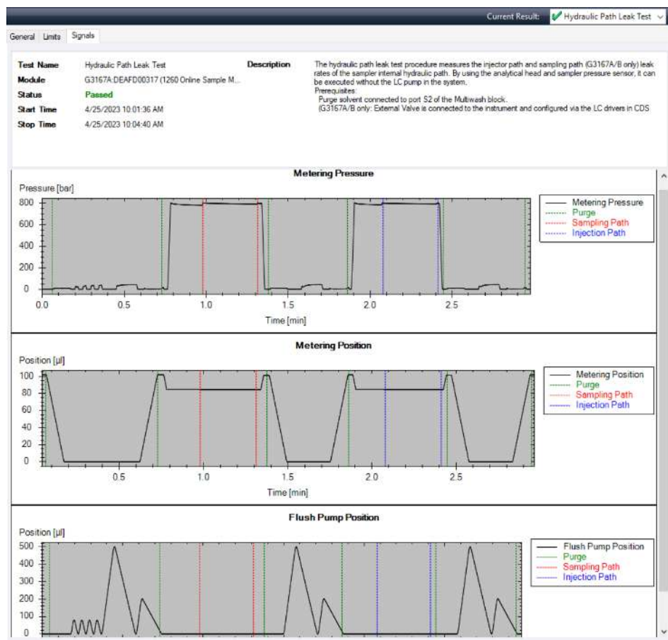
Figure 42: Hydraulic Path Leak Test passed
