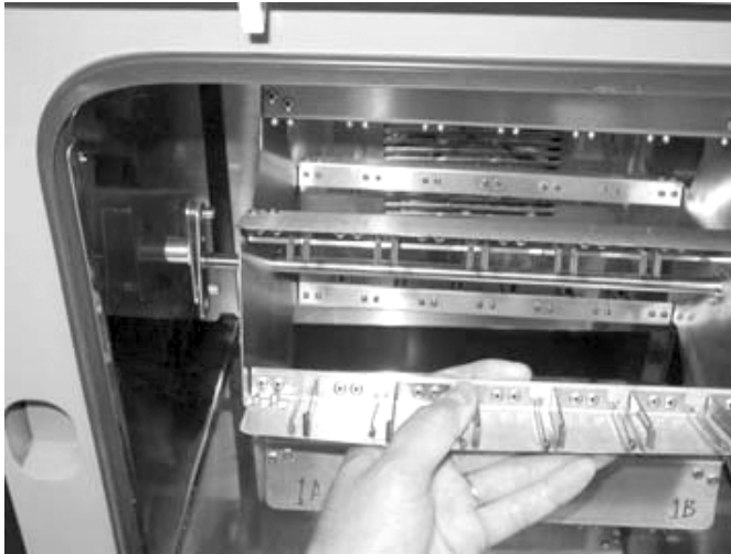
Figure 3 Attaching the rotator to the drive shaft coupling
