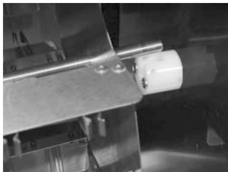
Figure 4 Inserting the rotator shaft into the rotator shaft support bushing.
