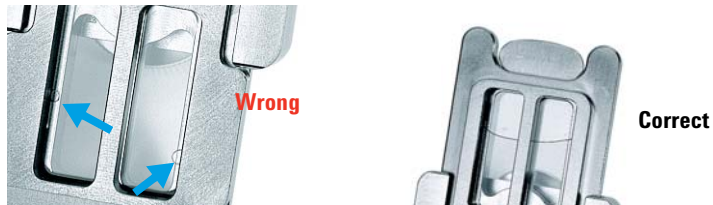
Figure 1 The slide on the left shows stray or stationary bubbles, which must be removed before hybridization. The slide on the right shows a single large mixing bubble, which moves freely around the chamber when rotated. Multiple bubbles are acceptable, as long as they move freely when you rotate the chamber.
