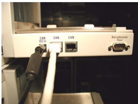
Figure 29 Connections to the Automation Interface and Well-plate Sampler
