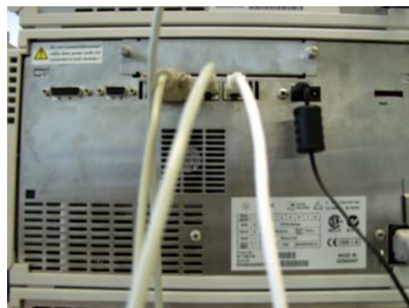
Figure 29 Connections to the Automation Interface and Well-plate Sampler
