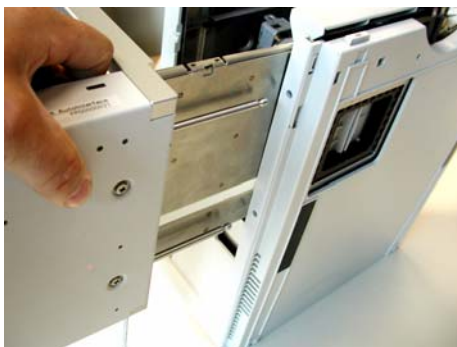
Figure 10 Moving the Automation Interface into the autosampler
