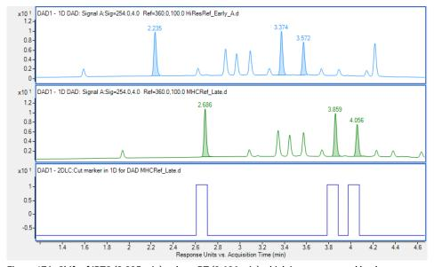
Figure 176 Shift of IRTS (2.235 min) to later RT (2.686 min) which is compensated by the system
