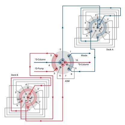
Figure 38 Schematic representation of the ASM 2D-LC Valve (G4243A) in countercurrent flow.
