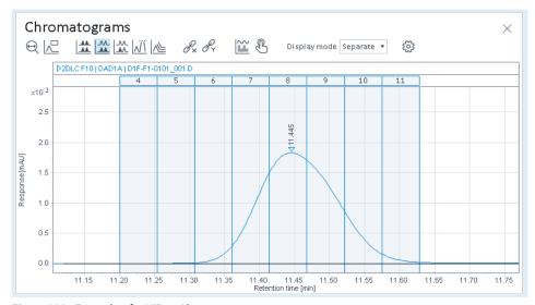
Figure 228 Example of a HiRes Chromatogram
