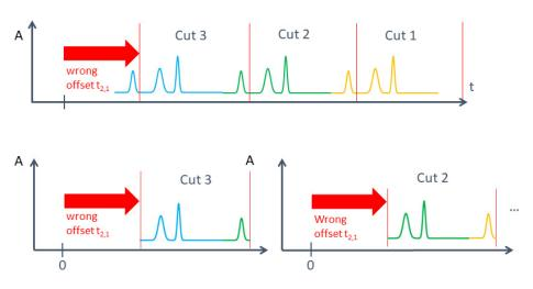
Figure 250 Wrong signal cutting in case of a wrong transfer time
