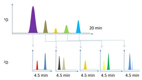
Figure 6 Example of a Multiple Heart-Cutting experiment with several cuts
