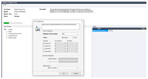
Figure 307 System Pressure Test for the 2D-LC 1290 binary pump
