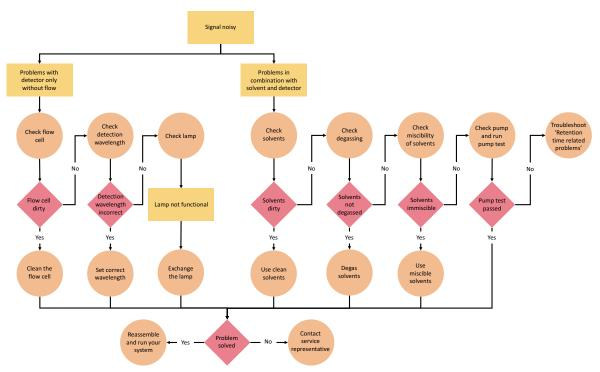
Figure 316 Example for a strategy to eliminate issues related to signal noise in 2D-LC instruments
