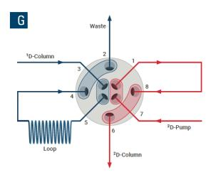
Figure 48 Setup G. Single Heart-Cutting Configuration as Single Sample Loop Setup
