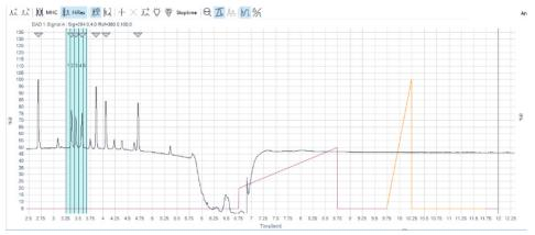
Figure 170 Example of High-Resolution Sampling (5 cuts) with only one analytical gradient for all cuts
