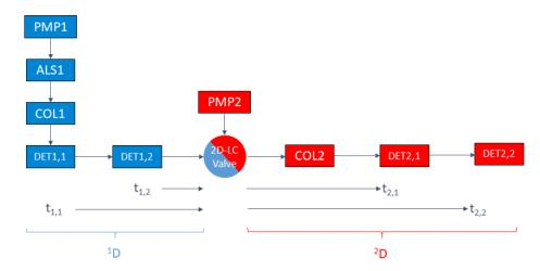
Figure 247 2D-LC Flow path diagram with transfer times
