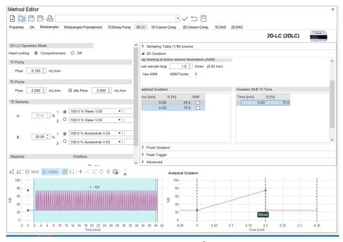
Figure 293 Method setup shallow gradient to improve the <sup>2</sup>D separation
