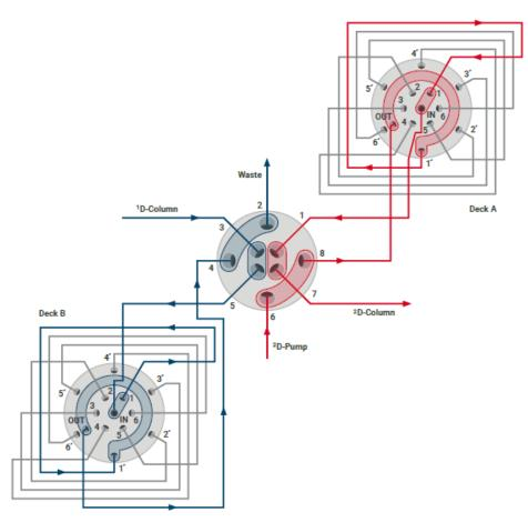
Figure 5 Standard 2D-LC valve (G4236A) with MHC 1300 bar (counter current)
