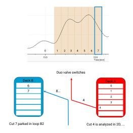
Figure 13 High-Resolution Parking principle with cut 7 parked in loop B2
