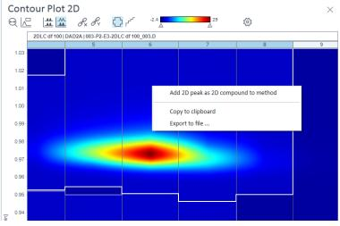
Figure 265 Add 2D peak as 2D compound to method in Contour Plot 2D
