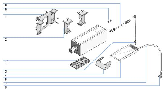
Figure 320 Parts for 1290 Infinity II Valve Drive
