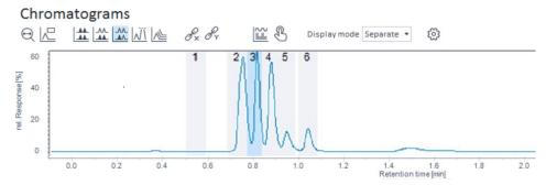
Figure 23Analysis of pesticides using a HILIC separation with high organic solvent composition in <sup>1</sup>D
