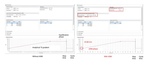
Figure 181 Programming the <sup>2</sup>D gradient table (example)
