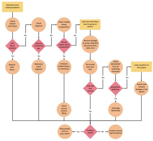
Figure 313 Example for a strategy to eliminate issues related to retention time in 2D-LC instruments
