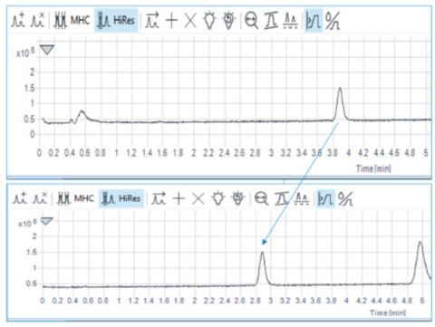
Figure 153 Example of a loaded Q-TOF signal with shift volume set to 0  $\mu$ L compared Q-TOF signal with shift volume set to -100  $\mu$ L
