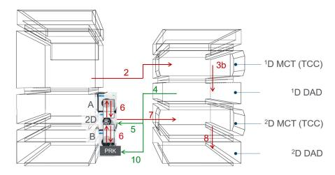
Figure 43 Setup B. Recommended setup if the instrument contains separate MCTs/ TCCs for <sup>1</sup>D and <sup>2</sup>D columns.
