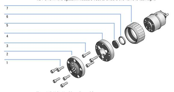
Figure 317 Valve Head Parts (example)
