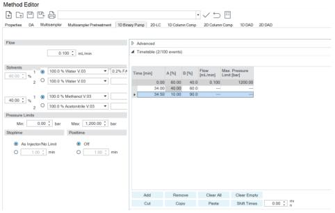
Figure 290 1D Binary Pump method
