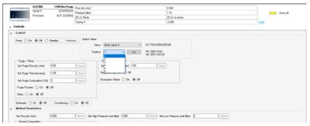
Figure 302 Example of a 2D-LC instrument with a selected MHC valve (Deck A)
