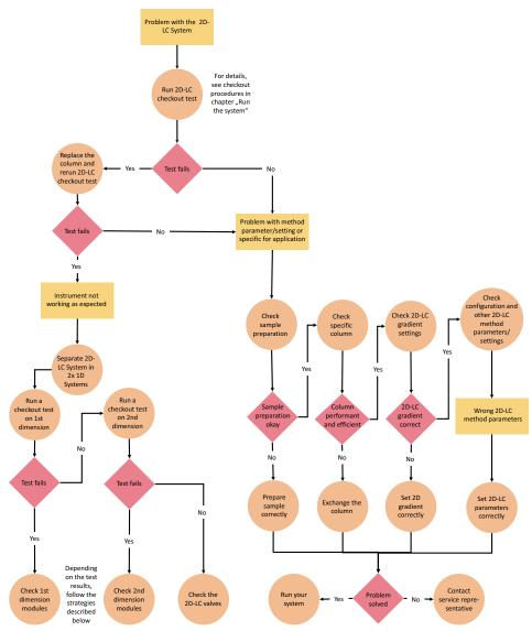
Figure 309 Example for a strategy to identify the application method or instrument as root cause for issues in 2D-LC chromatography
