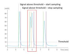
Figure 147 Chromatogram with Threshold and Slope settings
