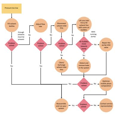
Figure 311 Example for a strategy to eliminate issues related to too low pressure in 2D-LC instruments
