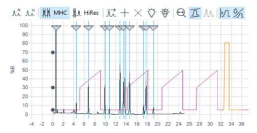
Figure 155 Preview of the display of the analytical <sup>2</sup>D gradient in purple and the flush in orange
