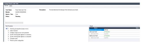
Figure 305 Pump Head Leak Test for the 2D-LC 1290 binary pump
