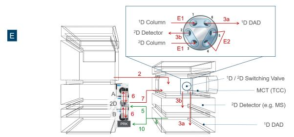
Figure 46 Setup E. Recommended setup for the  $^1\mathrm{D}/^2\mathrm{D}$  switching valve.
