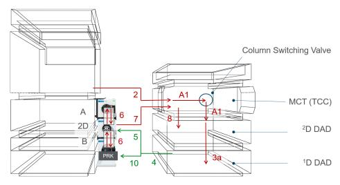
Figure 42 Setup A. Recommended setup if a column switching valve (for example 6-position/14-port InfinityLab Quick-Change Valve) is used. For a InfinityLab 2-position/6-port Quick-Change Valve, adapters A1 are not necessary.
