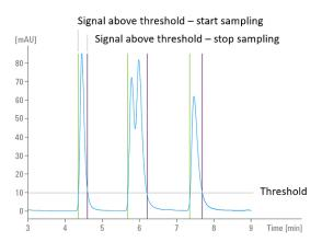
Figure 145 Chromatogram with Threshold line
