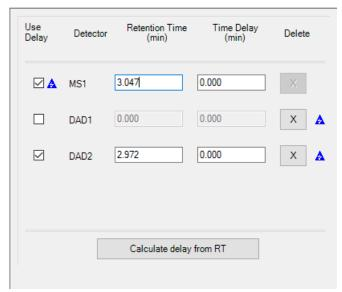
Figure 210 Retention Time Value for Peak1 (MS RT 3.047min and DAD2 2.972 min)
