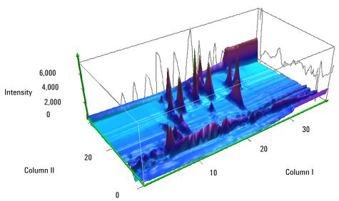
Figure 278 3-Dimensional display of the separation of the 26 compound standard mixture. The first dimension separation takes 40 minutes and each second dimension separation takes 39 seconds. The back side shows a generated first dimension chromatogram and gives the impression which peaks are coeluting and separated in the second dimensions.
