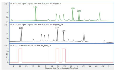
Figure 175 Shift of IRTS (2.686 min) to earlier RT (2.234 min) which is compensated by the system
