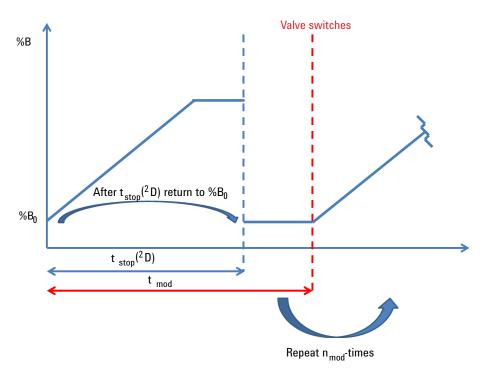
Figure 15 Characteristics of LCxLC
