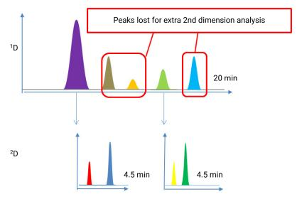
Figure 4 Example of lost peaks in Single Heart-Cutting
