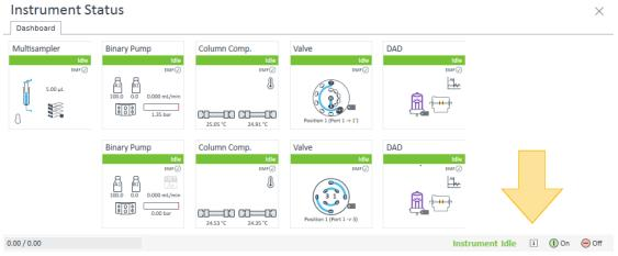
Figure 117 Instrument Status view
