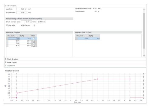
Figure 182 Optimizing separation using a lower percentage of B for the ASM and column equilibration phase (example)
