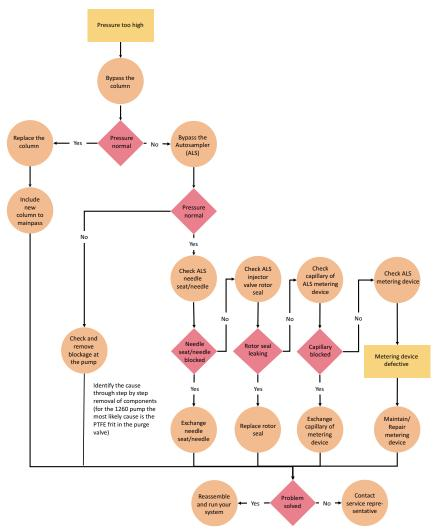
Figure 310 Example for a strategy to eliminate issues related to too high pressure in 2D-LC instruments
