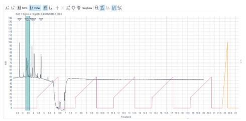
Figure 169 Example of High-Resolution Sampling (5 cuts) with 5 analytical gradients
