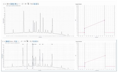
Figure 150 Preview panel with loaded reference chromatogram (top) and with threshold settings and detected peaks in the loaded reference chromatogram (bottom)
