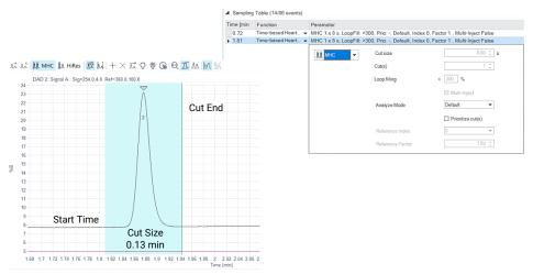
Figure 8 Time-based mode MHC
