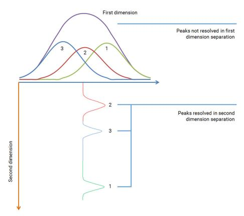
Figure 326 Peak capacity relationship between peak capacities of orthogonal first and second dimension
