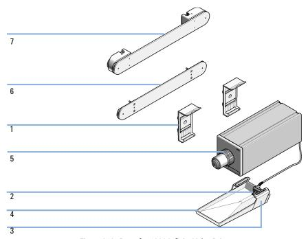
Figure 319 Parts for 1290 Infinity Valve Drive
