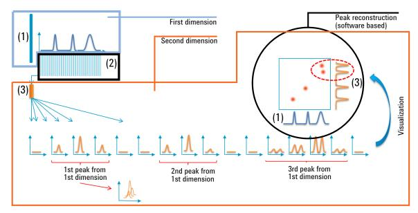
Figure 332 Principle of 2D-LC (example for LCxLC): Effluent of first column (1) is sampled (2) and injected to second column (3). Peaks of second column separation are detected and reconstructed.
