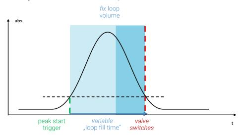
Figure 20 Peak triggering concept (signal falls below threshold or slope)
