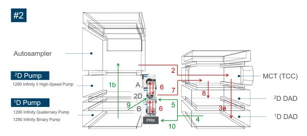
Figure 40 Stack Setup #2. Recommended setup if the <sup>1</sup>D pump is a 1290 Infinity Binary Pump or a 1290 Infinity Quaternary Pump.
