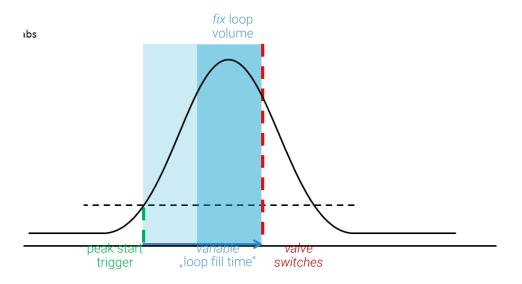
Figure 19 Peak triggering concept (elapsed sampling time)
