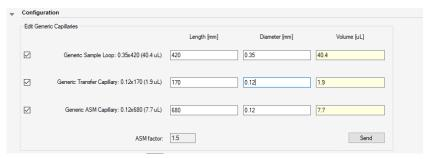
Figure 300 2D-LC generic capillaries configuration
