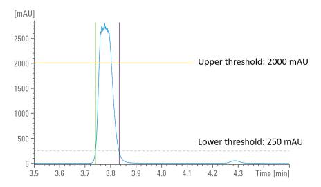
Figure 148 Chromatogram with upper and lower threshold
