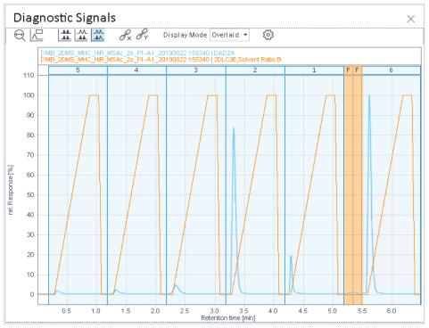
Figure 246 Diagnostic signals: Detector response and solvent ratio
