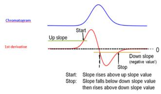
Figure 146 Example for triggering the slope of the detector
