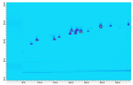
Figure 292 Example of separation after comprehensive 2D-LC analysis
