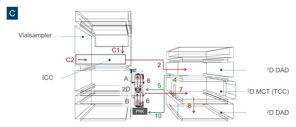
Figure 44 Setup C. Recommended setup if <sup>1</sup>D column is hosted in an Integrated Column Compartment (ICC).
