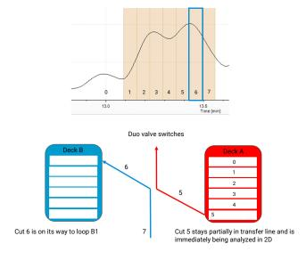
Figure 11 High-Resolution Parking principle with cut partially in transfer line
