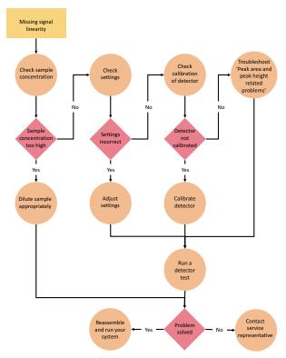
Figure 314 Example for a strategy to eliminate issues related to missing signal linearity in 2D-LC instruments
