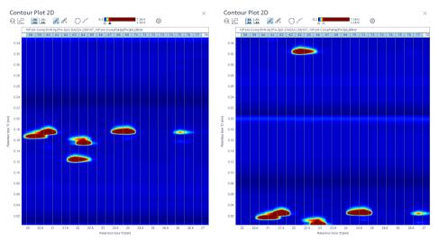
Figure 251 Left image: aligned signal using the correct transfer time; right image: not aligned.
