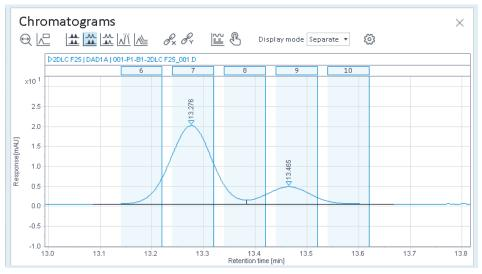
Figure 227 Example of a MHC Chromatogram
