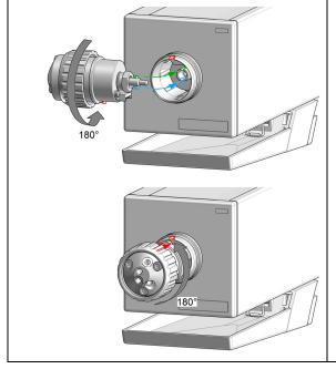
When the outer pin is locked into the groove, manually screw the nut onto the valve head.
