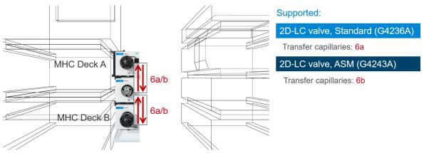
Figure 35 Schematics of a Multiple Heart-Cutting (MHC) Configuration with supported valves and transfer capillaries.
