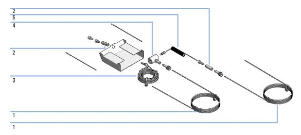
Figure 325 Pressure release kit, parts
