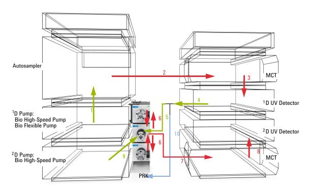
Figure 55 Recommended setup if both bio pumps are Infinity II modules or the <sup>2</sup>D pump is a 1290 Infinity Bio High-Speed Pump
