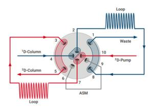
Schematic representation of the Bio 2D-LC ASM Valve without MHC in concurrent flow
