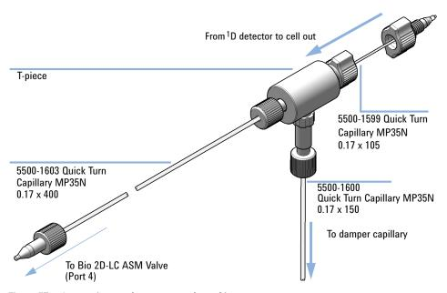
Figure 57 Connections to the pressure release kit
