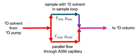
Figure 31 Principle of active solvent modulation (schematic view)
