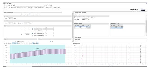
Figure 334 Shifted gradient mode with increase of start-%B
