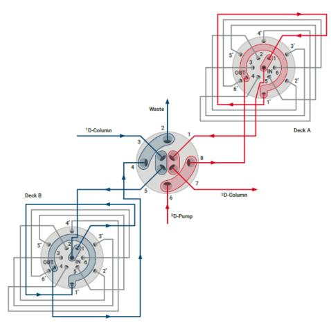
Figure 37 Standard 2D-LC valve (G4236A) with MHC 1300 bar (counter current)
