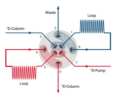
Figure 36 Schematic representation of the Standard 2D-LC Valve (G4236A) in concurrent flow.
