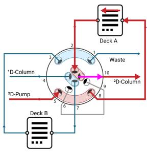
Figure 29 Operating principle with sample loop flow path
