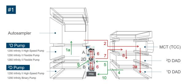
Figure 39 Stack Setup #1. Recommended setup if both pumps are Infinity II modules or the <sup>2</sup>D pump is a 1290 Infinity Binary pump.
