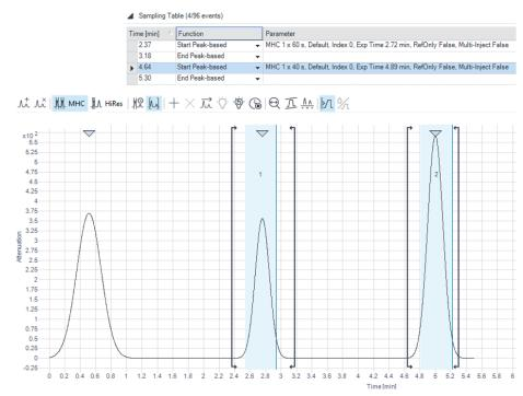
Figure 161 Two selected peaks in peak based mode and corresponding peak-based sampling table
