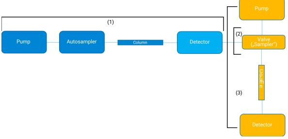
Figure 331 Diagram of instrumentation for 2D-LC
