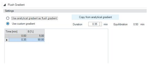
Figure 142 Flush Gradient table view
