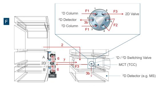
Figure 47 Setup F. Recommended setup for the  $^1D/^2D$  switching valve without  $^1D$  detector.
