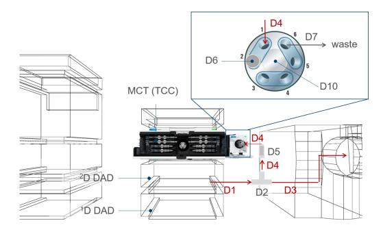
Figure 56 Recommended setup of a MS diverter valve
