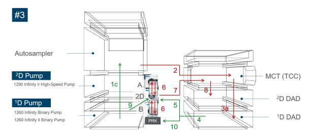
Figure 41 Stack Setup #3. Recommended setup if the <sup>1</sup>D pump is a 1260 Infinity or 1260 Infinity II Binary Pump.
