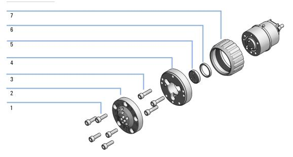
Figure 321 Valve Head Parts (example)
