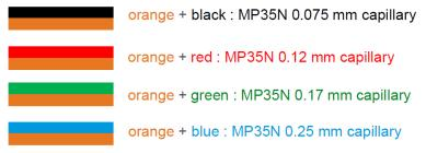
Figure 324 Color code for biocompatible capillaries
