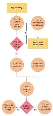
Figure 315 Example for a strategy to eliminate issues related to drifting signal in 2D-LC instruments
