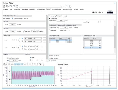
Figure 295 Method of stepwise shifted gradients
