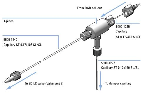
Figure 49 Connections to the pressure release kit
