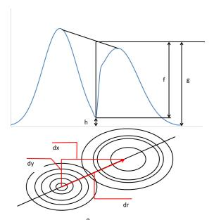
Figure 328 Diagram of <sup>2</sup>D resolution measurement: Slice for resolution (top) and 2-dimensional contour plot (bottom)
