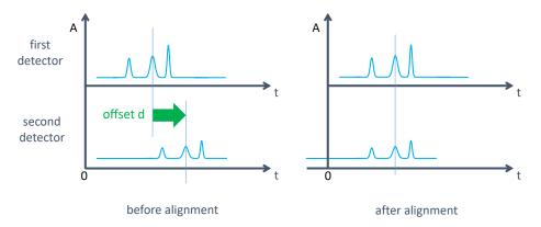
Figure 252 Signal alignment using the transfer time between detectors
