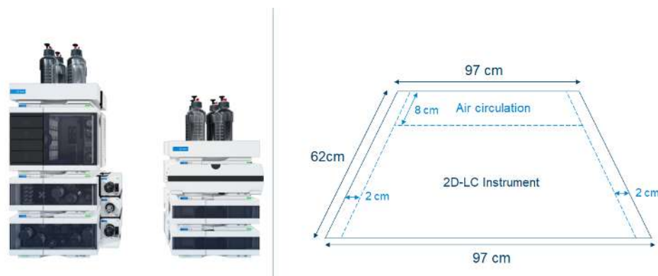
Figure 26: Left: Recommended stack configuration for the 1290 Infinity III 2D-LC System. Right: Bench space requirements of the 1290 Infinity III 2D-LC System.
