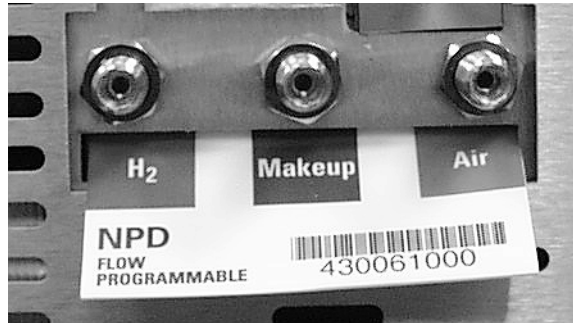
Figure 5. Gas line connections
