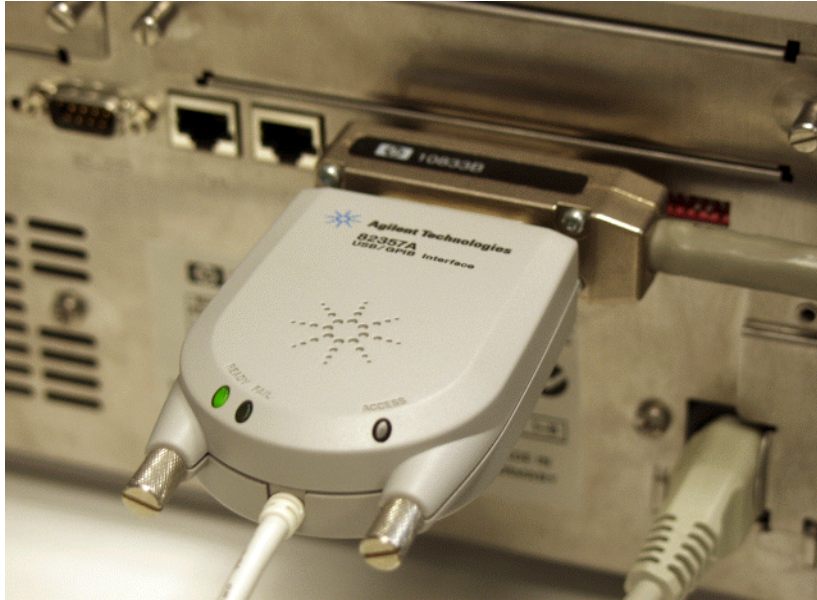
Figure 39 82357 USB-GPIB Interface on e.g. 8453 spectrophotometer
