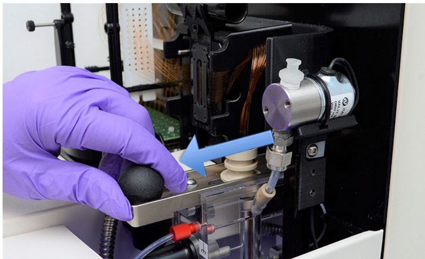
Figure 54 Instrument top compartment – capillary reservoir connector slide
