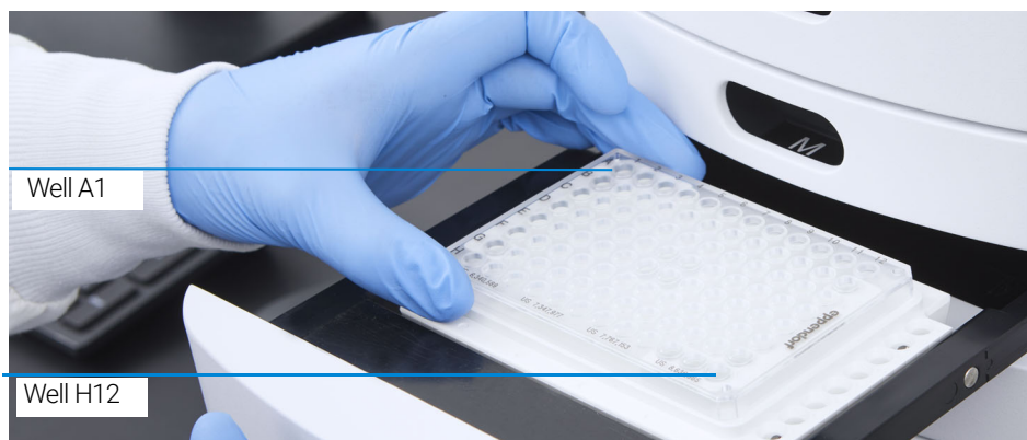
Figure 9 Proper orientation when loading 96-well marker and sample plates for a 12-capillary system
