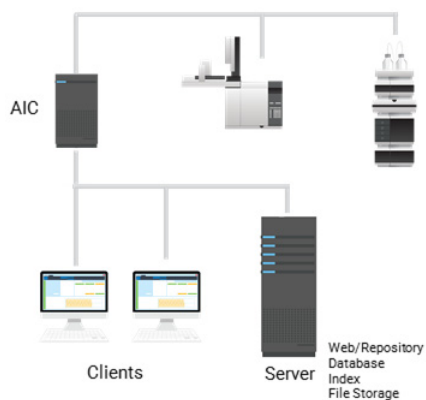
Figure 1. OpenLab Server/ECM XT all-in-one system architecture
