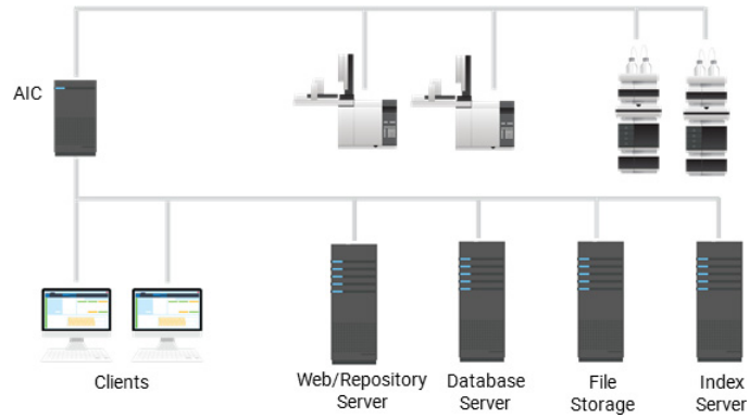
Figure 3. Four-server system architecture
