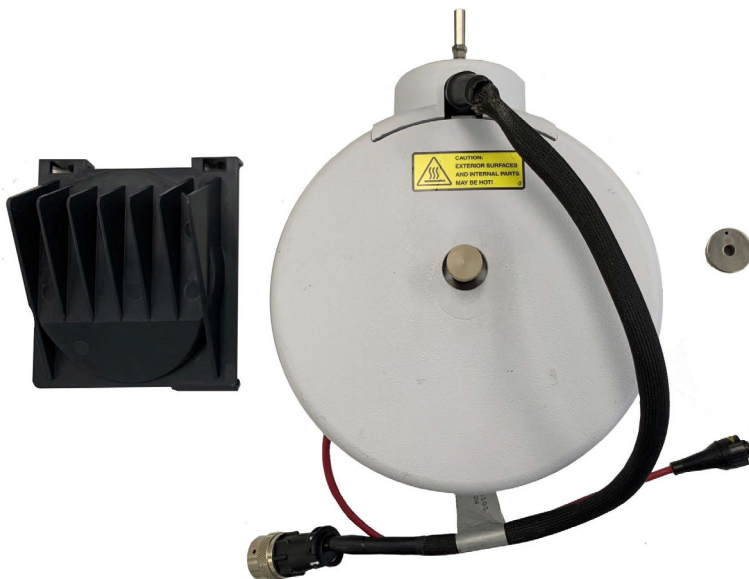
Figure 16. APCI cover, ion source, and spray shield
