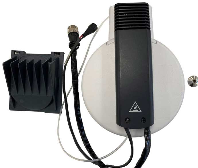
Figure 15. AJS ESI cover, ion source, and spray shield
