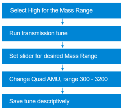
Figure 25. High-mass tune and calibration (6545XT)
