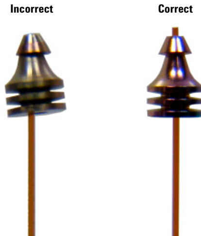
Figure 7 Incorrect and correct swaging symmetry
