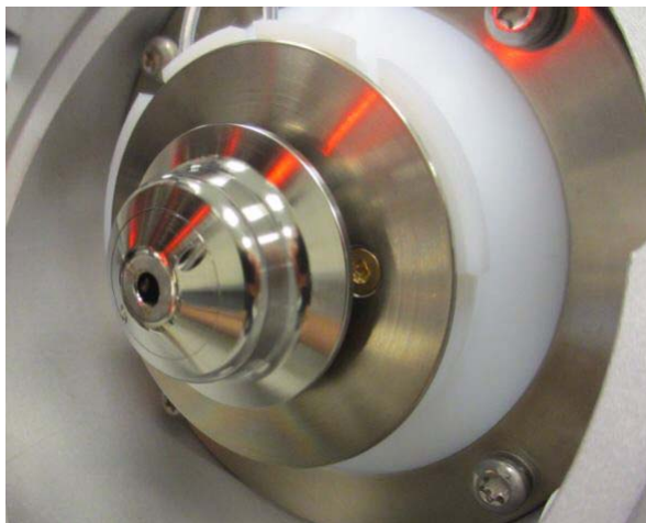
Figure 9 Installed spray shield assembly. (Multibore vortex spray shield shown)
