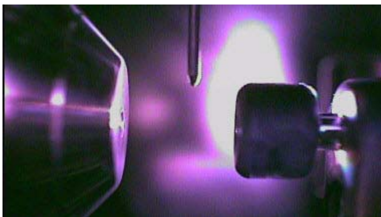
Figure 25 Needle safely inserted midway between the spray shield and Counter Electrode .
