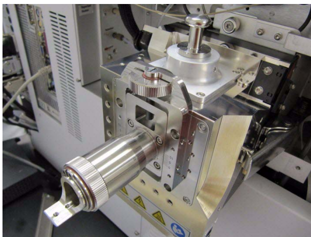
Figure 34 Nanospray Slide Assembly installed for Inline Horizontal Orientation .
