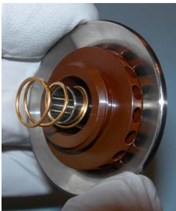
Figure 8 Contact spring installed onto spray shield assembly
