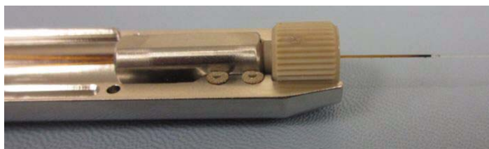
Figure 18 Analytical column attached to the needle, seated in the Needle Sleeve Assembly.
