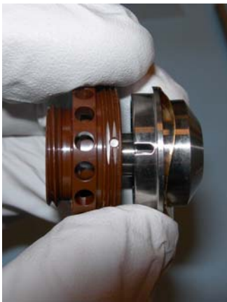
Figure 6 Gas diverter pin aligns with the spray shield groove
