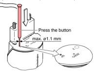
For changing the threshold value, push the <ZERO> button and keep it depressed. The threshold keeps changing from the current value (ramp) until the button is released or until the limit of the setting range is reached.
