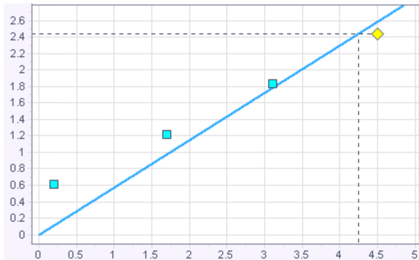
Figure 91: Force calibration curve through the origin
