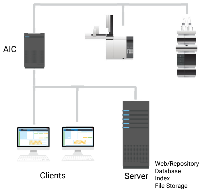
Figure 2 Client/Server System, 1-server system
