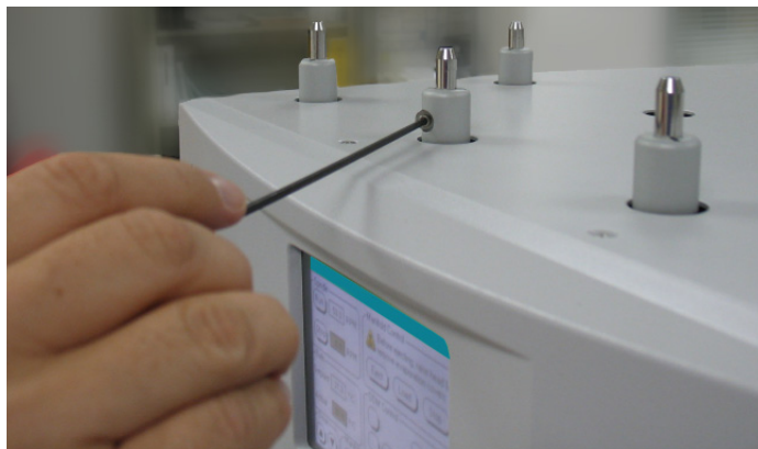
Figure 22 Tightening the Shaft Locking Collar
