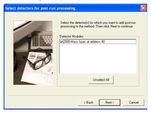
Select Channel 1=MS Data, Standard MS Reports and MS Data Handling in the Create sections for post-run processing dialog and then click Next.
