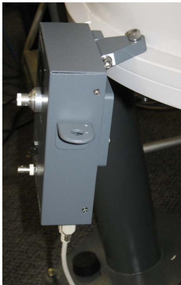
Figure 2 Mounting the Tachometer module
