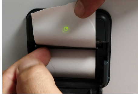
Figure 50. Inserting a Thermal New Paper Roll
