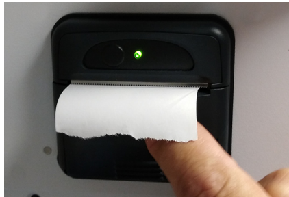
Figure 51. Closing the Printer Chamber
