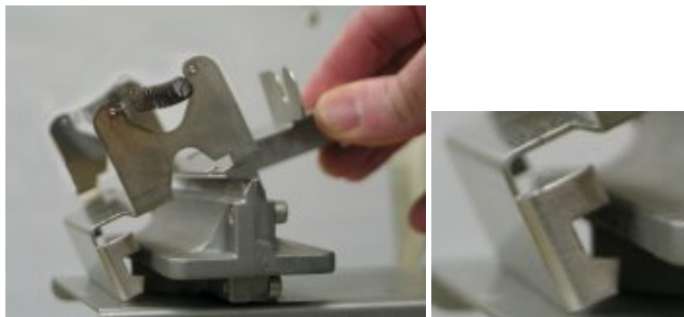
Figure 2 Tube holder pulled forward with cut-outs hooked around burner edge
