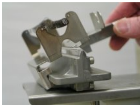
Figure 3 Tube holder pulled forward with cut-outs hooked around burner edge
