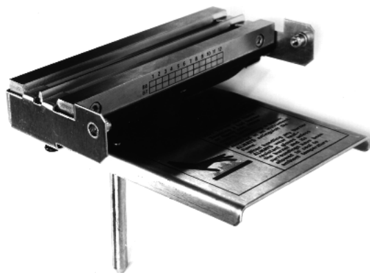
Figure 8 Mark V burner with the adaptor installed
