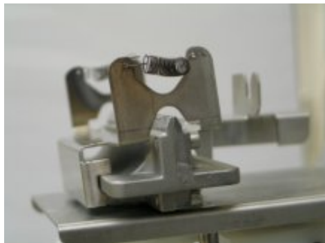
Figure 4 Lowering the tube holder into position on the Mark 7 burner
