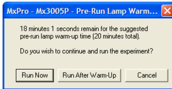
**Important** *Do not open the instrument door during the run. When an experiment is running, the upper LED on the instrument front is in blinking mode. Opening the door while the instrument is running will abort the run.*
