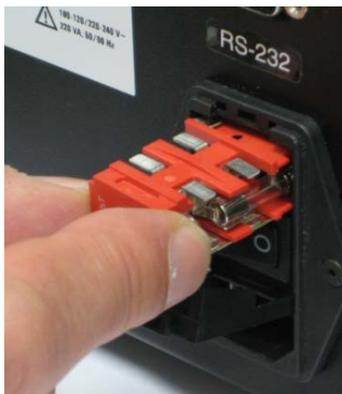
5. Replace the cover on the fuse box. Verify that the correct voltage label is visible through the cover.
