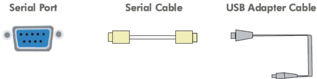
**Figure 1** Appearance of the serial port, serial cable and USB adapter used to connect the instrument to the PC. Note that this cable configuration is only required when using a PC that does not have a serial port or when using the PC's USB port to allow Multiple Instrument Control from a single PC.
