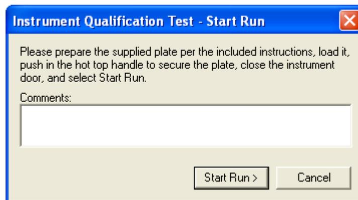
4. Verify that the Perfect Fit frame shipped with the instrument has been removed from the thermal block area. (See the *Sample Loading* section for more information.) Load the plate in the thermal block, verifying the correct orientation (well A1 in the top, left corner), and then close and latch the thermal block lid to secure the plate. Close the instrument door, and then click **Start Run**.
