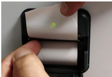
Figure 50. Inserting a Thermal New Paper Roll
