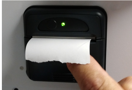
Figure 51. Closing the Printer Chamber
