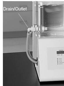
**Figure 1.** Water Bath Connections
